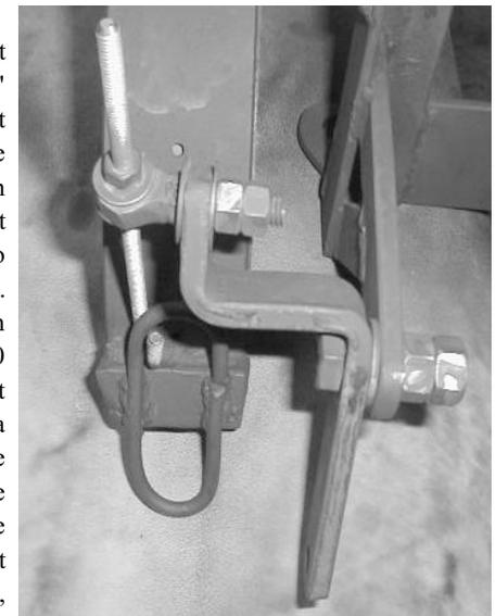
**Fig.7:Control arm (from side)**
